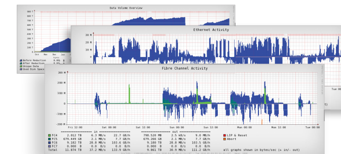
Quantum management tools provide details of internal appliance operations and single-console views across all of a user's disk and tape systems. They reduce management time, streamline performance tuning, accelerate troubleshooting, and provide trend analysis information for proactive decision-making that maximizes system value.
