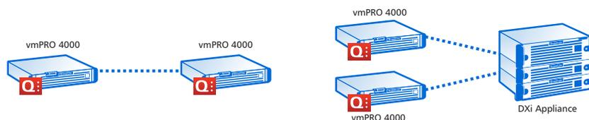
*For automated DR protection, vmPRO solutions replicate deduplicated data to other vmPRO systems. In distributed deployments, multiple devices can replicate data to a DXi appliance in a data center.*
